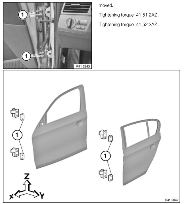
Adjust rear door in transition to front door (Y) by fitting shims.
